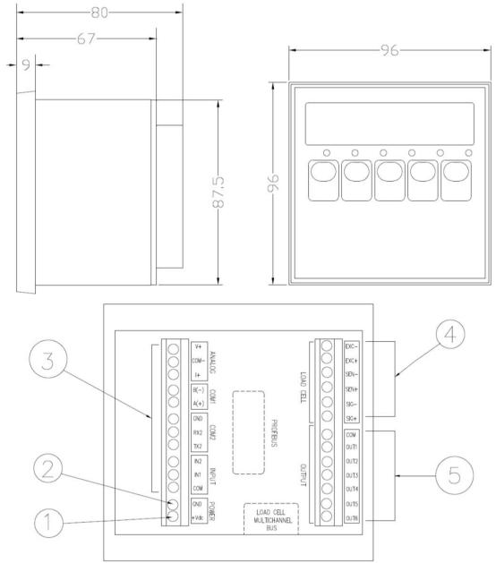
1 and 2 power supply (12 to 24Vdc) 3 connection RS232 and 485
