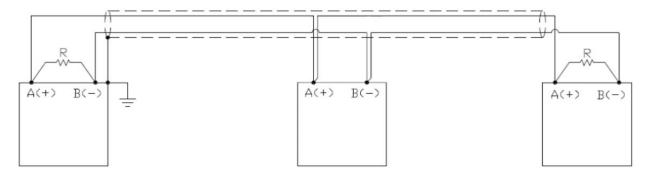
On the RS485 network normally one connects 2 termination resistors of 120 Ohm (shown with "R" in figure). Only on the 2 devices which are at the end of the network.
