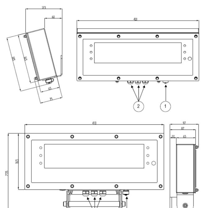
1 : gland for power supply connection 110/220Vac 2 : gland for serial communication connection
