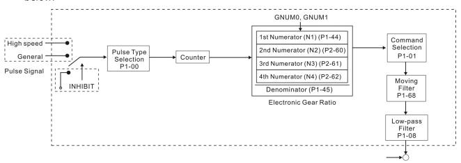
Using parameter P1-01 can select P mode. Electronic gear ratio can be set in P modes to set proper position revolution. ASDA-B2 series servo drive also provides low-pass filter, which are used whenever the motor and load need to be operated more smoothly. As for the information of electronic gear ratio, and low-pass filter, please refer to the following sections 6.2.3 and 6.2.4.
