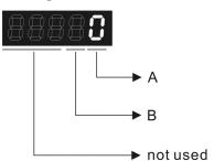
A: Analog monitor outputs polarity
