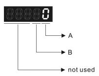
A: Analog monitor outputs polarity B: Position pulse outputs polarity
