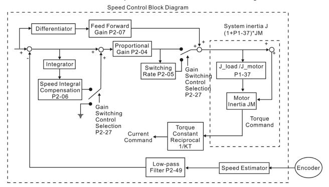
There are two turning modes of gain adjustment: Manual and Auto modes. The gain of ASDA-B2 series servo drives can be adjusted by using any one of three tuning modes.
