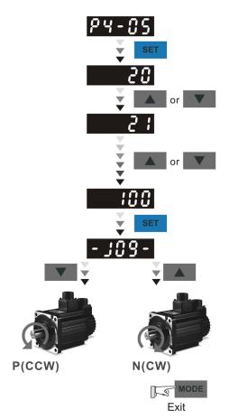
Pressing key and the servo motor will run in P(CCW) direction. After releasing UP key, the motor will stop running.
