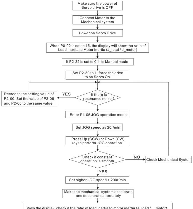
View the display, check if the ratio of load inertia to motor inertia ( $J_load/J_motor$ ) become a fixed value after the motor accelerates and decelerates alternately many times and then decide the gain adjustment method.
