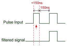
When this pulse frequency is less than 150 ns, this signal will be regarded as a low-level pulse and two input pulses will be regarded as one input pulse.
