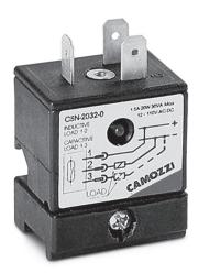
It is designed so that it can be fixed directly on the tie-rod by means of two screws which assure the position longitudinal to the cylinder axle; and with a third screw for the anti-rotation positioning. The three terminals are indicated by the numbers 1, 2 and 3 and enable the following connections to be made (see the scheme).
