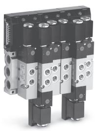
This Plug-In system, realized with electropneumatically operated valves Series 3, G1/8 port, is delivered completely assembled and tested. It allows the mounting of up to 22 valve positions (with two SUB-D 25 RIGHT and LEFT connectors).
