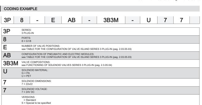
3P8-EAB-3B3M-U77 = Valve island with 6 positions equipped with 3 Solenoid valves Cod. B and 3 Cod. M, SUB-D connector on the LEFT.
