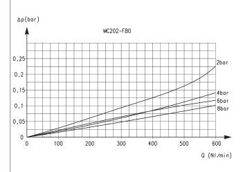
Flow diagram for model: MC202-FB0  $\Delta P$  = Pressure drop
