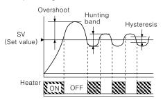
As like above picture, the control value is up and down by set value, it is called Hunting. And Overshoot is occurred at initial point when just power on.
