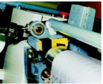
Workpieces of different shape and size and of ferritic or nonferritic materials will induce the sensor to generate a specific output signal upon attenuation, depending on the typical characteristics and shape of the workpiece. Thus it is possible to distinguish between different kinds of materials.
