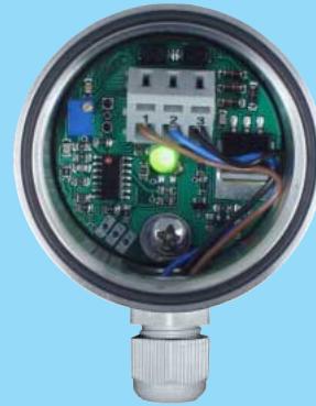
Inside view with LED switching status indicator nwm-141.w, nwm-041.w
