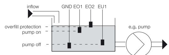
The vessel is filled via the inflow pipe. When the maximum level (EO1) is reached, the pump is switched on. As soon as the minimum level electrode (EU1) loses contact to the medium the pump stops. The overfill electrode (EO2) prevents an overflow of the vessel in case of an error.
