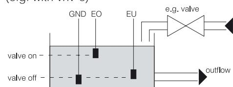
The medium is continuously taken out of the vessel via the outlet in the bottom. As soon as the minimum electrode (EU) loses contact to the medium, the valve in the inflow pipe is opened and the vessel gets filled again. When the medium reaches the maximum electrode (EO) the valve is closed again and the filling stops.
